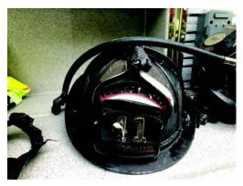
Heat damage to a helmet worn by an MOFD firefighter responding to the Orinda house fire Photo courtesy MOFD
