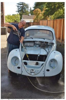
Hays Englehart, Beetle rehab project leader, powerwashes front bay, from which spare tire had been removed. All of the mechanical-repair work was done at his home in Moraga.
