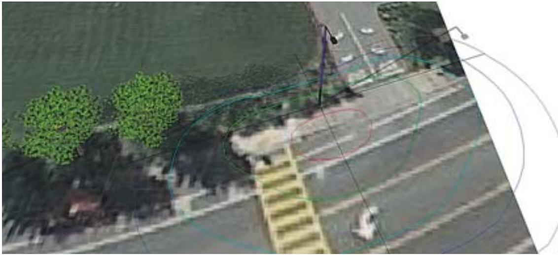
Solar lighting shading analysis at 10 a.m. on Corliss Drive
