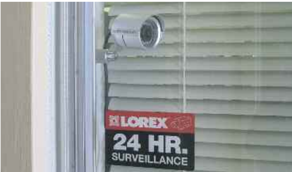
Small cameras are popular security devices that can be integrated into home networks, so that any motion or pictures can be sent to a cell phone.
