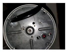
The bottom of garbage disposals have a circuit breaker button than can be pushed when the breaker trips. Photo provided
